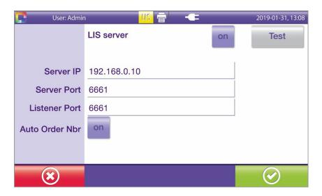
After setting up the Solana with an IP address for its network connection, configure the LIS interface settings.
